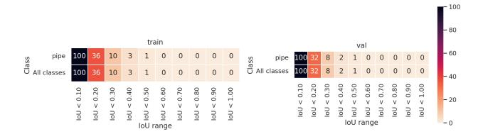
The distribution of the box Intersection over Union (IoU) with respect to other boxes in the sample. The heatmap shows the percentage of boxes that overlap with IoU in range [0..T] for each class. Intersection of all boxes is considered (Regardless of classes of corresponding bboxes).
