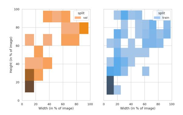
These heat maps illustrate the distribution of bounding box width and height per class. Large variations in object size can affect the model's ability to accurately recognize objects.
