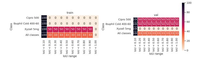
The distribution of the box Intersection over Union (IoU) with respect to other boxes in the sample. The heatmap shows the percentage of boxes that overlap with IoU in range [0..T] for each class. Intersection of all boxes is considered (Regardless of classes of corresponding bboxes).
