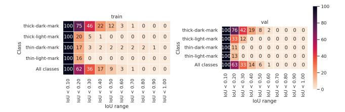
The distribution of the box Intersection over Union (IoU) with respect to other boxes in the sample. The heatmap shows the percentage of boxes that overlap with IoU in range [0..T] for each class. Intersection of all boxes is considered (Regardless of classes of corresponding bboxes).
